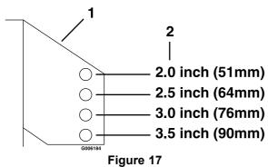
For cutting heights above 3.5 inches (90 mm) use the bottom hole. The rollers will still be effective against scalping.
